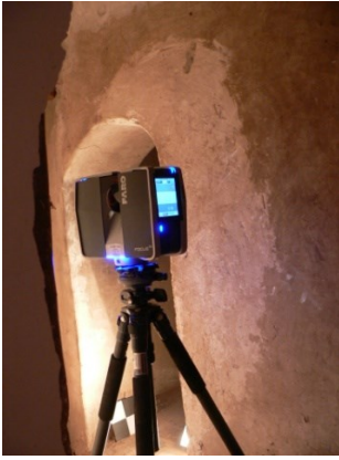
Fig. 10 Laser scanner in the very low-rise rooms of the hammam in kasbah Taourirt
