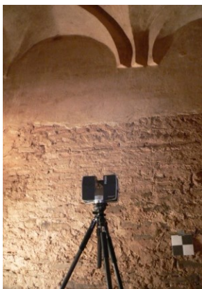
Fig. 6 3D laser scanner in the main room of the hammam in kasbah des Caids of Tamnougalt
